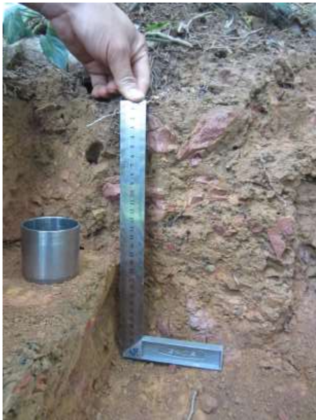
Collecting soil samples in a fixed volume ring. Photo: Suzanne Stas
