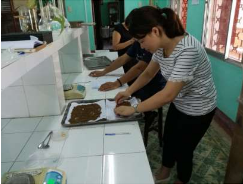
Preparing the soil samples for oven-drying in the lab. Photo: Suzanne Stas
